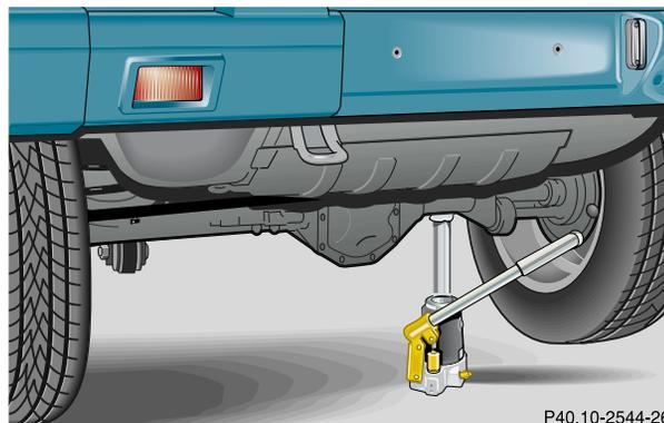
Position vehicle jack in the correct position under the axle housing when raising the vehicle.
