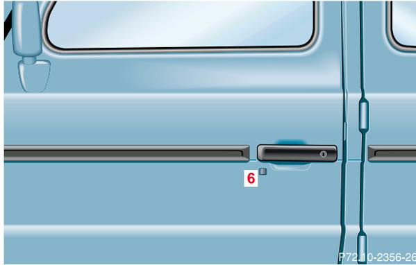
6 Infrared receiver at the driver's door
