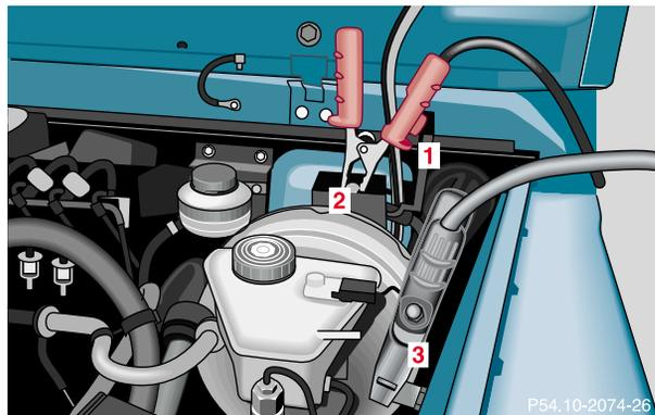
Jump starting terminals are located in the left side of the engine compartment.
