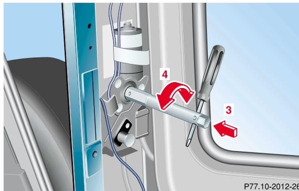
2. Place socket wrench (3) on hexagon. The sliding/pop-up roof can be moved in the desired direction (4) by turning the socket wrench. To open sliding/pop-up roof, turn clockwise. To close sliding/pop-up roof, turn counterclockwise.
