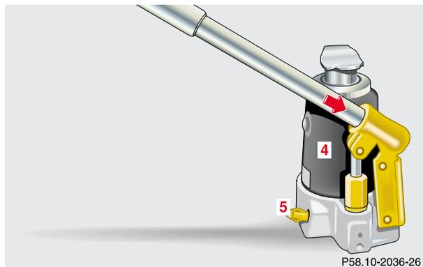
Insert pump handle in direction of arrow.
