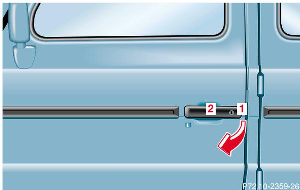
To open the door, press the lock cylinder (1) and pull on the door handle (2).
