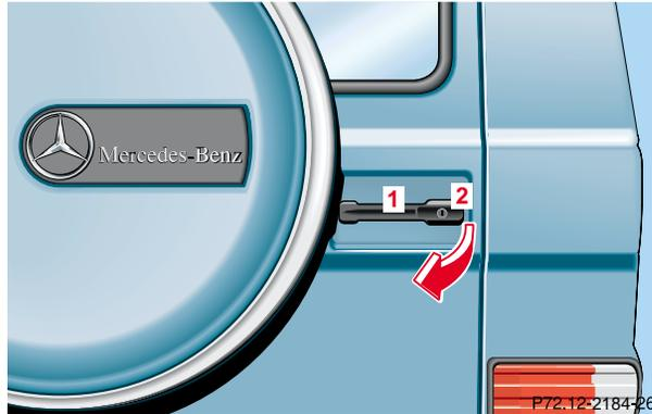
To open the tailgate, press the lock cylinder (2) and pull on the tailgate handle (1).
