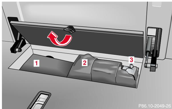
The first aid kit (1), vehicle tools (2) and jack (3) are located in the storage compartment below the rear seat bench.
