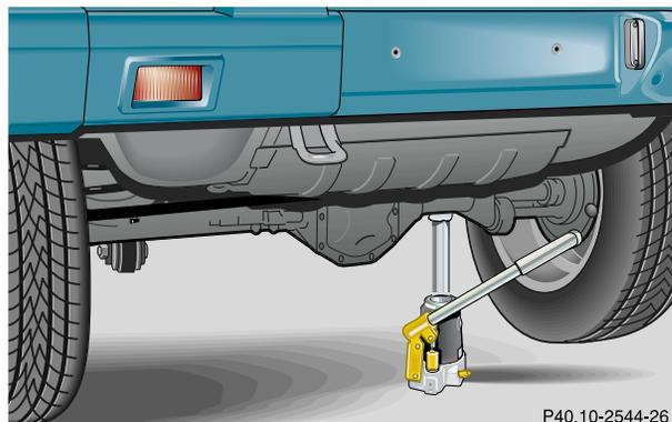
5. The jack must always be in a vertical position, even on slopes. Place jack under axle housing. Be certain the jack arm is positioned correctly under the axle housing.
