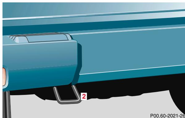
The rear towing eye (2) is located on the left side below the bumper.
