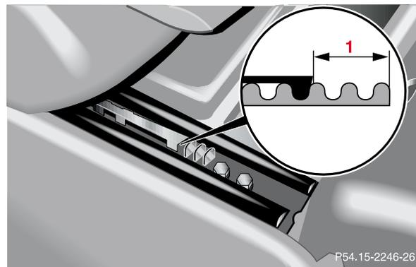
Remove both front end stops of front passenger seat tracks.
