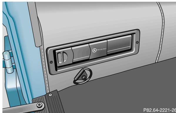
The CD-changer is located in the left side of the cargo compartment.
