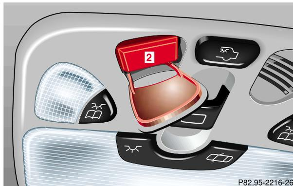
Press the SOS button (2) briefly. The indicator lamp in the SOS button (2) will flash until the emergency call is concluded. Wait for a voice connection to the Response Center.
