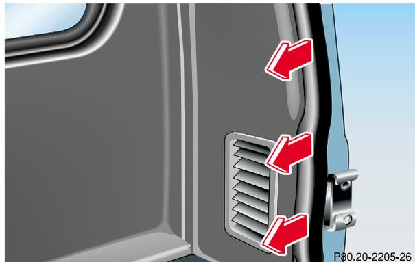
Remove edge molding and trim panel on right rear door pillar.
