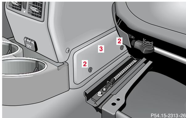
Unscrew mounting screws (2) and remove cover (3).
