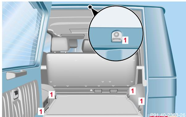
The anchorage rings (1) are located in the rear cargo compartment. Located on each side of the passenger compartment are two anchorage rings (for the rear outer seats) and one on the roof pillar above the tailgate (for the rear center seat).
