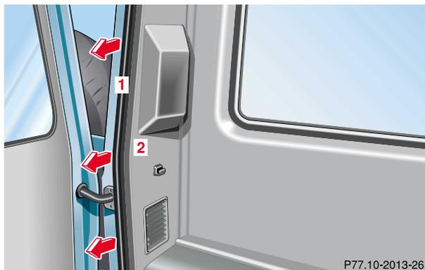
The sliding/pop-up roof can be opened or closed manually should an electrical malfunction occur. The sliding/pop-up roof drive is located behind the cargo area trim panel (2).
