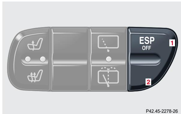
ESP control switch located in center console.
