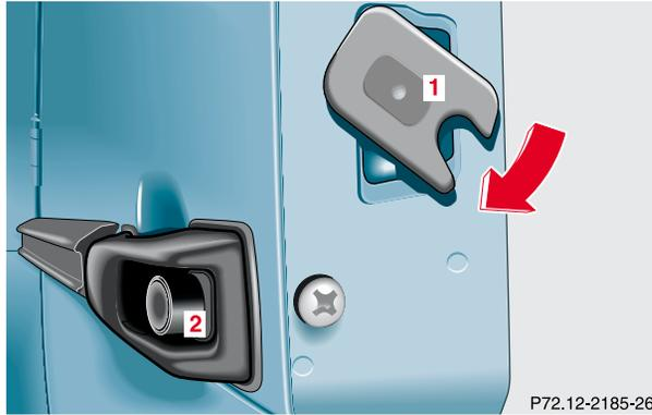
If the tailgate should remain open for a longer period of time, the cargo area lamps may be switched off separately from the rear compartment lamps. Press the door lock (1) down until it clicks into place (arrow).
