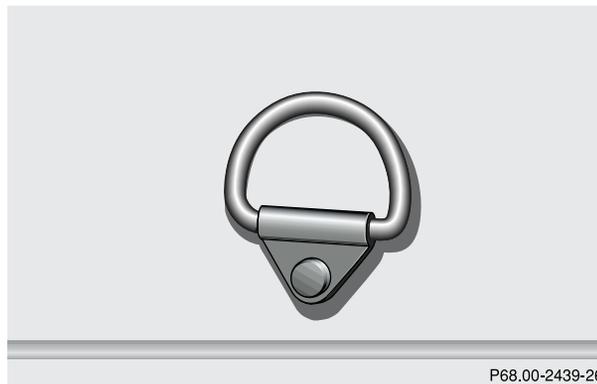
Carefully secure cargo by applying even load on all rings with rope of sufficient strength to hold down the cargo. The cargo area is provided with four tie-down anchors.
