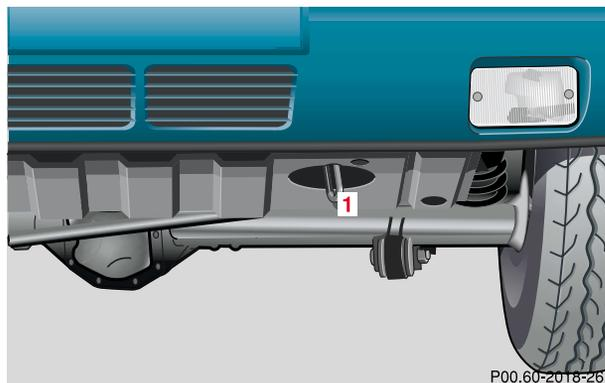
The front towing eye (1) is located on the left side below the bumper.
