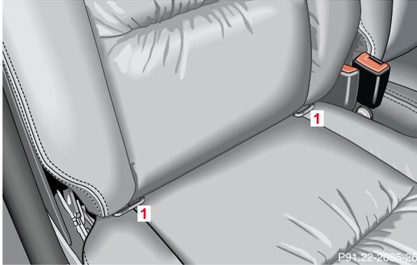
This vehicle is provided with two “LATCH” type mounts (at each of the outer rear seats) for the installation of a “LATCH” child seat having the matching mounting fittings.
