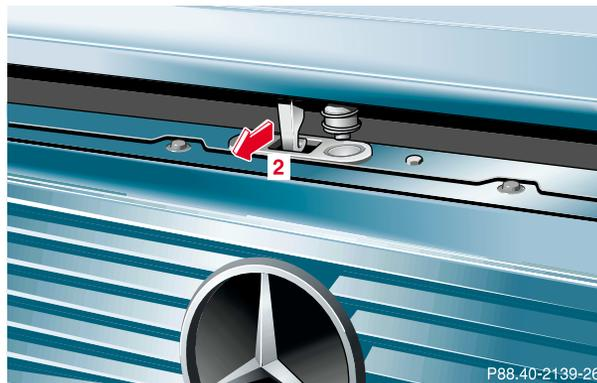
Lift hood up slightly. Pull safety hook (2) in direction of arrow and open hood.
