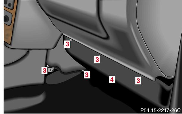
2. Unscrew mounting screws (3) and remove cover (4).
