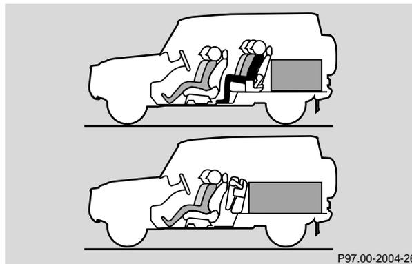
The total load weight including vehicle occupants and luggage/cargo should not exceed the vehicle capacity weight indicated on the certification label which can be found on the left door pillar.
