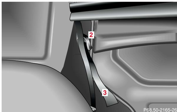
1. Engage partition net in holders (1). The lift tensioner (2) must point in driving direction (forward).
