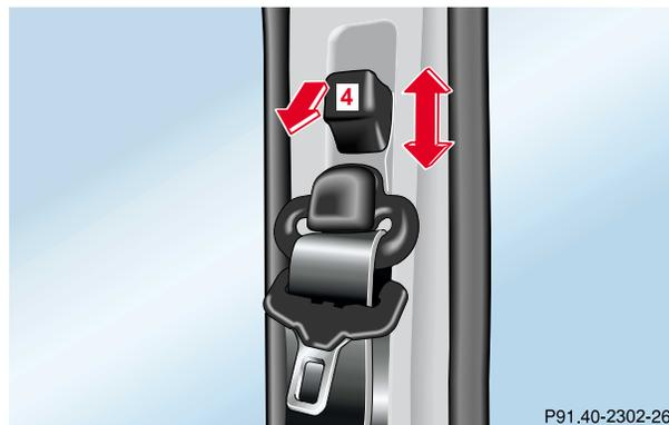
4 Button for belt outlet height adjustment
