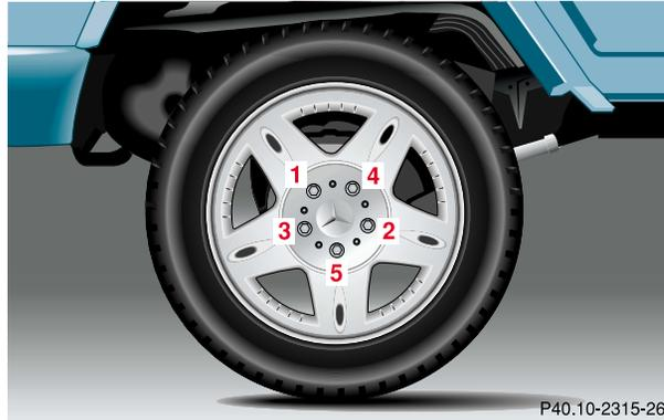
With the vehicle lowered to ground, tighten the five bolts evenly using the wrench. When tightening follow the sequence illustrated, until all bolts are tight. Observe a tightening torque of 97 ft.lb. (130 Nm).
