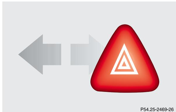
The hazard warning flasher can be activated either manually via the switch located in the center console, or it is activated automatically at the time an airbag is deployed.
