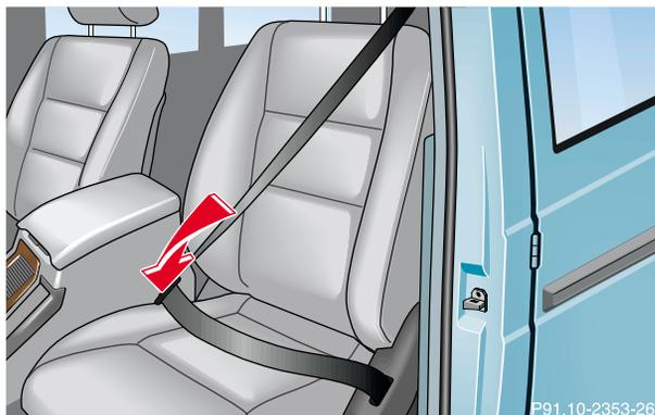
Tighten the lap portion to a snug fit by pulling shoulder portion up.
