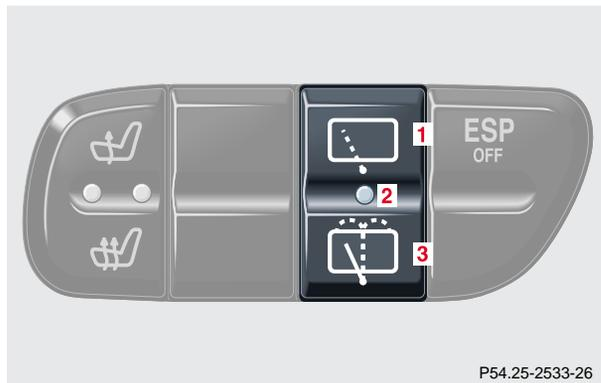
The rear window wiper/washer switch is located in the center console.
